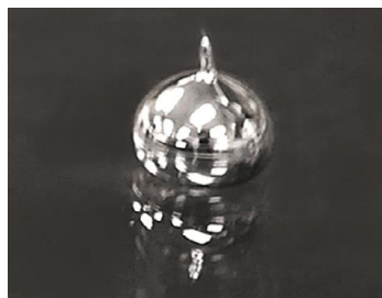
Figure 6. Drop of Galinstan evidencing the high surface tension
