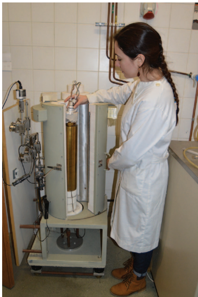
Transient hot-wire instrument for humid air thermal conductivity for advanced adiabatic compressed air energy storage (solving a problem open since 1928)
