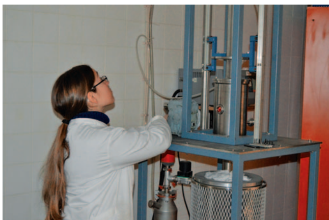
High temperature oscillating-cup viscometer for new car engine molten alloys
