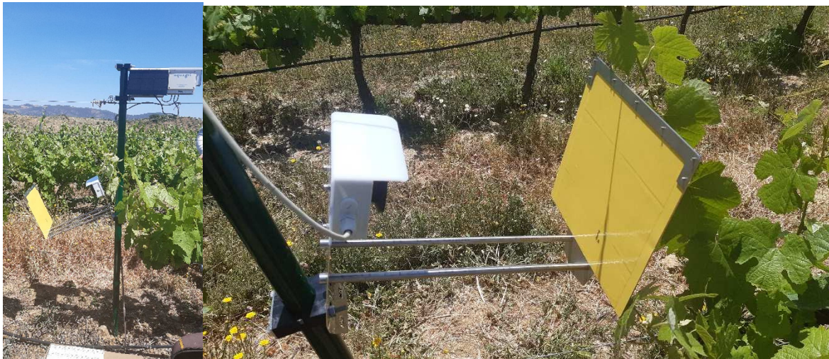
Figure 1. iSCOUT@COLOR TRAP: general perspective (left); camera and yellow sticky trap (right).
