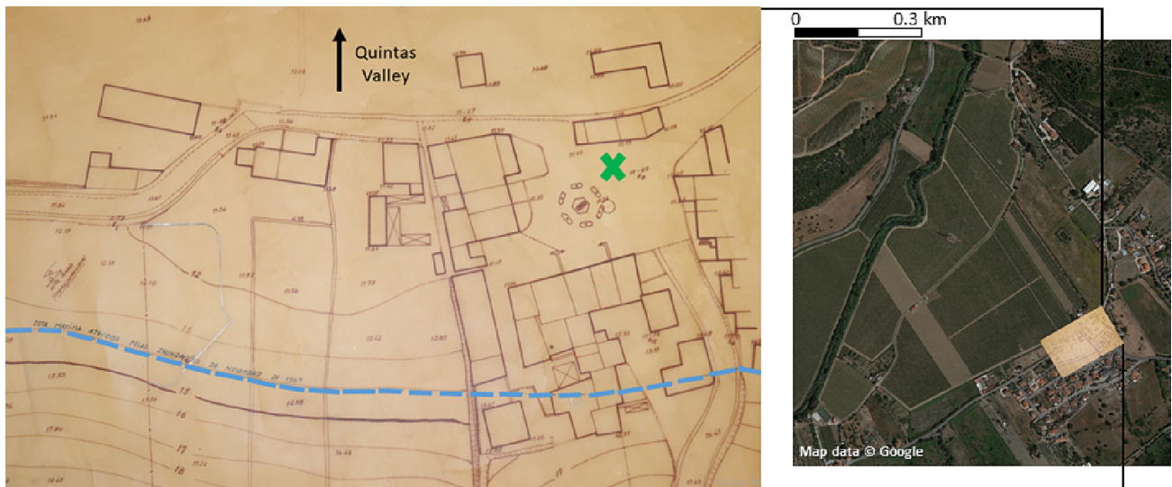
Fig. 2. The left panel shows a topographic map of the centre of Quintas village in 1967 (see the lower grey rectangle in Fig. 1c to visualize its location within the context of Quintas valley), including a line indicating the maximum water level reached in the November 1967 flood (approximately coincident with the 14-m topographic isoline). The original flood line was highlighted in dashed blue to facilitate the visualization. The main square of Quintas, located in the upper right part of the figure (marked with a green cross), was considered as a benchmark for the flood in Quintas village. This point presents an approximate level of 11.25 m, which means that water depth reached approximately 2.75 m in this point. The direction where Quintas valley is located is also indicated. The photograph was taken by the authors within the framework of the official consultation to the historical archive of the municipality of Vila Franca da Xira. The right panel shows the area of Quintas village represented on the map. Map data © Google Satellite (accessed: December 2022).
