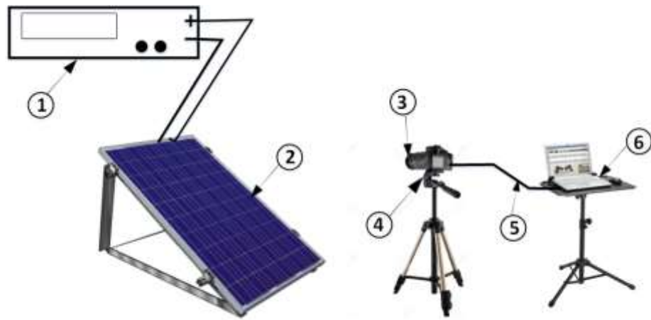
Figure 1: The proposed Electroluminescence setup, the setup consists of the (1) power supply, (2) PV module, (3) bandpass filter, (4) digital camera, (Nikon D40 with a 18-55mm f/3.5-5.6G ED II lens) (5) USB cable (5), and (6) PC.
