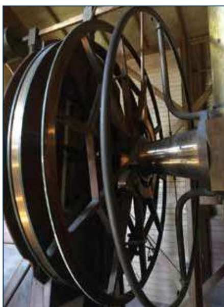
Fig. 7 Two close-ups showing (a) the hand circle at the axis, for rapid movements, and (b) the arm with a pressure screw on the side of the hand circle. Photograph by the author:
