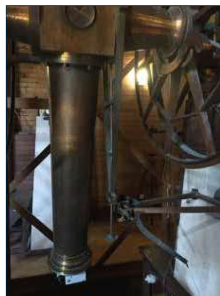
Fig. 7 Two close-ups showing (a) the hand circle at the axis, for rapid movements, and (b) the arm with a pressure screw on the side of the hand circle. Photograph by the author:
